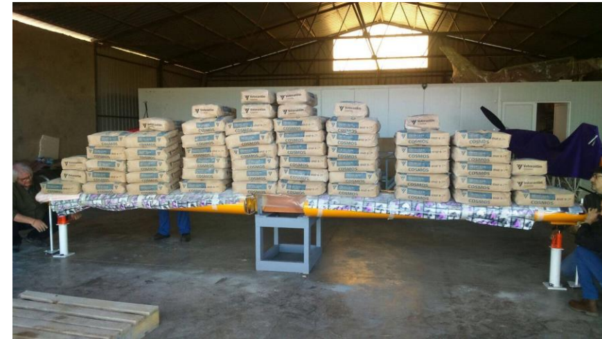
Static Load test- 6g's at 1,212 lbs. (7,272 lbs)
