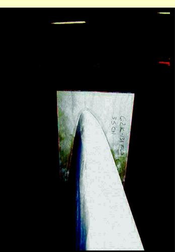
I have to finish sanding the leading edge so I stood the wing up on end to make the work easier. A quick check with the LE templates indicated that the leading edge was amazingly close to the design profile. The wing was most accurate from the root to the flap/aileron junction i.e. the planform break. The leading edge of the outer third of the wing deviated the most in that the nose (the 4 inches from LE) of the airfoil was too flat on top and bottom.
