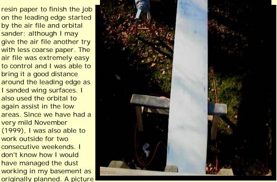
of the bottom of my sanded wing follows. The white areas are areas covered by thin gelcoat. All remaining gelcoat was examined with a 10-power scope to insure no crazing was evident.
