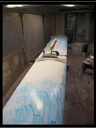
I use the air file to knock the high points off the paint (just about to the bottom of the orange peel) and then hand sand with a two-foot bar sander to remove the remaining blue. I also immediately sanded the spoiler area to see if I had any coverage or fit problems.
