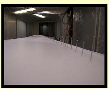
I painted the entire wing in one session using a setup, which allowed the surfaces to be painted flat, reducing the potential for runs. This was pretty easy because I
