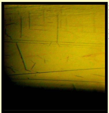
A magnified (10x) contrast enhanced picture of my leading edge crazing follows. This will be sanded down to the fiberglass surface. The airfile made the more lateral scratches in the upper area of the picture.
