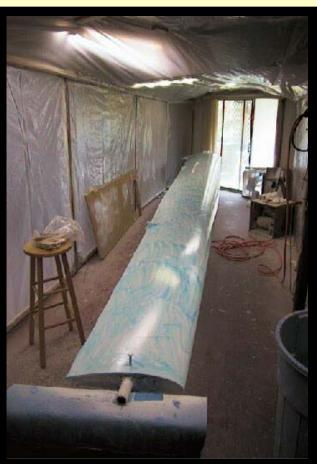
The paint dried with the typical orange peel. I then applied a mixture of thinned dope over both wing surfaces to disclose sanding progress. You simply have to sand until the blue is gone.
