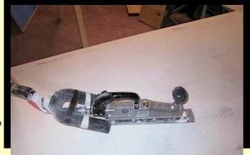
blade. The nozzle sucks the loose material off the surface and also does a good job pulling dust out of the air around the tool. Suction is supplied by large (low noise) shop vac; the shop vac hose
