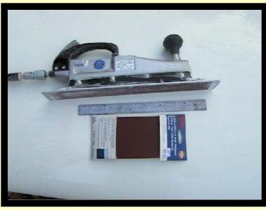
fiberglass. The 60-grit paper seems to rip the gelcoat off without touching the
